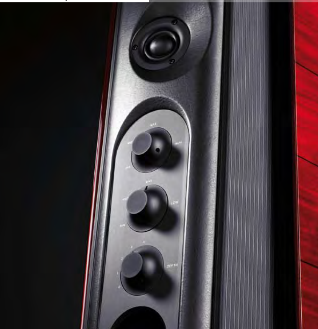
The controls allow to adjust the bass and treble levels and also the proportion of the rear diffuse radiator (Depth) which is silent in the 0 setting.
